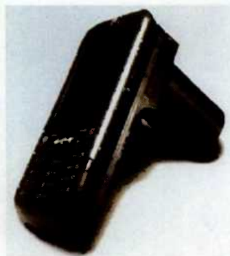
Photo 2—The cell phone microscope uses an internal app to analyze the photo it takes of a blood sample.
