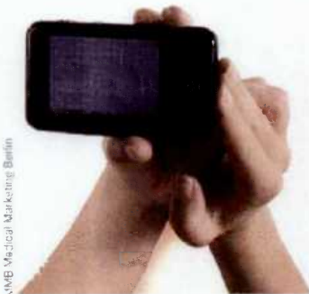
Photo 1—This cell phone performs an on-the-spot EKG. A new model that can also register body temperature and blood pressure is expected to receive FDA approval this year.
